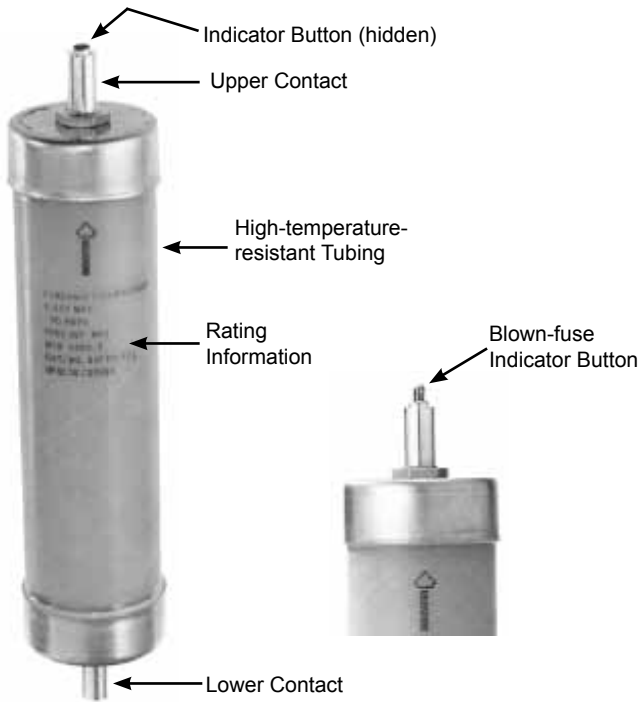
Eaton's Cooper Power Systems X-Limiter™ Full-Range Current-Limiting Fuse
