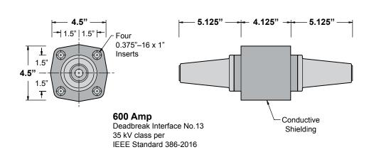
1.25" Dia. Tin-Plated Aluminum Conductor Tapped 0.625"–11 x 1.25" Deep (both ends of conductor)
