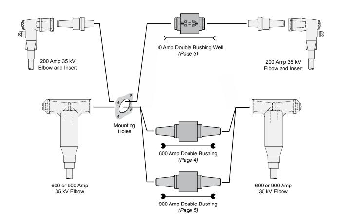
**Elliott Double Bushing Wells** are designed to accept IEEE Standard Fig. 3 Loadbreak Insert and Elbows.
