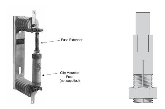
The Elliott Fuse Extender is designed to allow a clip mounted fuse to be placed in a mounting larger than the fuse. For example: a CM5-6 Fuse Extender will allow a Code 5 Fuse to fit switchgear with mountings designed for Code 6 Fuses.
